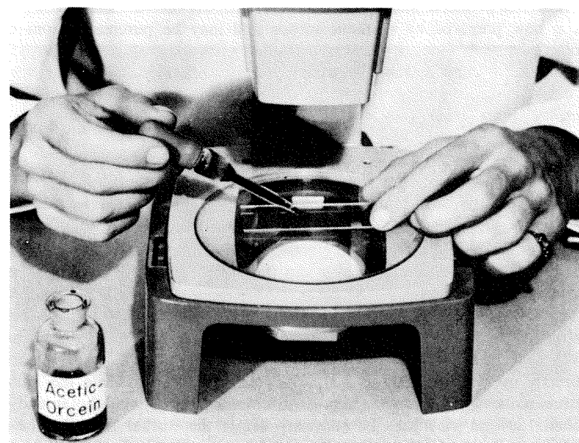
Fig. 12. Upper picture shows method of albuminizing slides. The salivary glands, after removal from the larva, are placed in a drop of aceto-carmin or acetic-orcein on the dried film of albumin, as shown in the lower picture.
