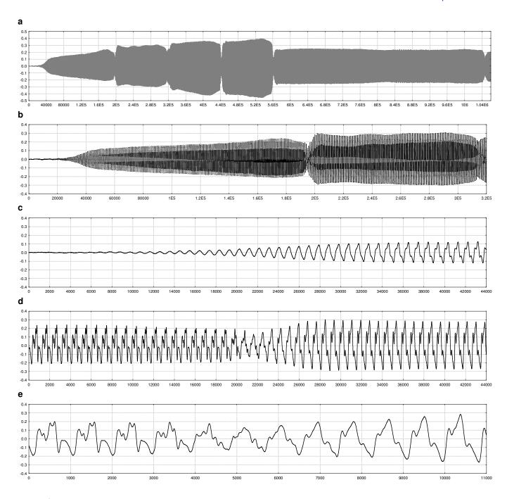
Figure 5 | Clarinet sound records. Abscissa – counts of ADC (192 kHz); ordinate – linear amplitude (24-bit original resolution). (a) The first measure (six notes, Fig. 4b) of the Fig. 4a; it contains slightly more than one million counts of the analogue-digital converter (ADC). (b) The first two notes. (c) The beginning of the first note. (d) The transition from the first note to the second one. (e) The same as (d), but shown with higher temporal resolution.
