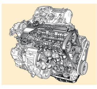
Figure 6 | VTEC engine. VTEC (Variable Valve Timing & Lift Electronic Control) engine was developed by Honda and introduced in 1989 in mass production. Note 3 cams (1 central & 2 peripheral) for each two valves.
