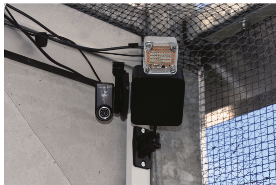
2D optical transmitter, IR emitter and video camera for observation mounted behind protective organic glass in the aviary
