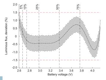
Solid black line shows luminous flux approximation error. It is below 1%. Dotted cloud around this line (±0.5%) represents discretization error caused by 1% step of power adjustment. The total error is always below 1.5% in the displayed range of battery voltages.
